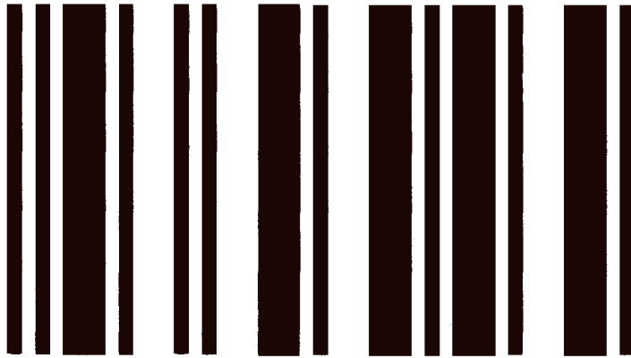
I2 of 5 symbol encoding the data “1991”.
