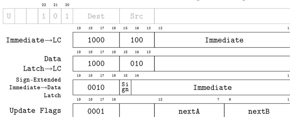
The FleetTwo implementation is likely to have an unarchitected “literal latch” at the on deck (OD) stage, which is loaded with the possibly-extended literal *at the time that the set instruction comes on deck*. This latch is then copied into the data latch when a set Data Latch instruction executes.
